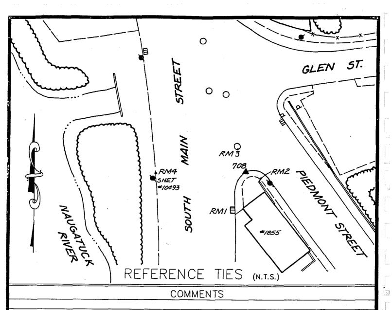
STATION #708: SET BRASS DISK IN CONCRETE CURB 24.5° ± NORTH OF NORTHWEST CORNER OF
