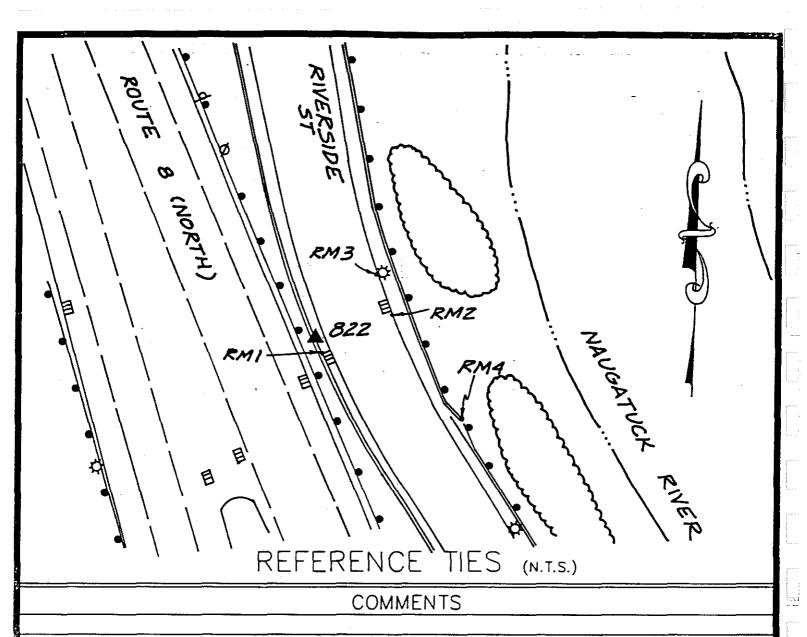
STATION #822: SET BRASS DISK IN CONCRETE CURB ON THE WEST SIDE OF RIVERSIDE ST., ABOUT 650' NORTH OF THE CENTERLINE OF FREIGHT ST., ABOUT 16' NORTH OF A CATCH BASIN ON THE WEST SIDE OF RIVERSIDE ST.
