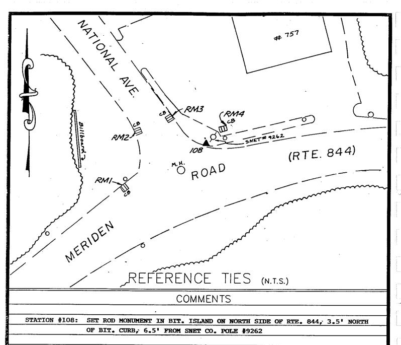
RM1: SOUTHWEST OF STATION - A 3/8" DRILL HOLE IN THE CONCRETE CURB OF CATCH BASIN
