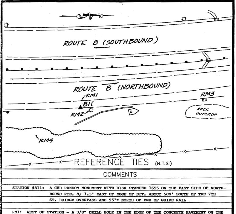
RM1: WEST OF STATION - A 3/8" DRILL HOLE IN THE EDGE OF THE CONCRETE PAVEMENT ON THE EAST SIDE OF NORTHBOUND RTE. #8
