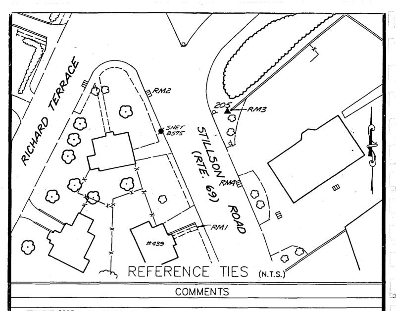
STATION #205: SET BRASS DISK IN LOWER PORTION OF A CONCRETE RETAINING WALL
