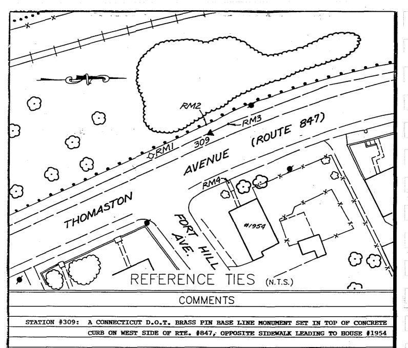
RM1: SOUTH OF STATION - TOP OF FIRE HYDRANT ON THE WEST SIDE OF RTE. #847, 1.5° WEST OF CONCRETE CURB AND 66° NORTH OF THE EXTENDED CENTERLINE OF FORT HILL AVE.
