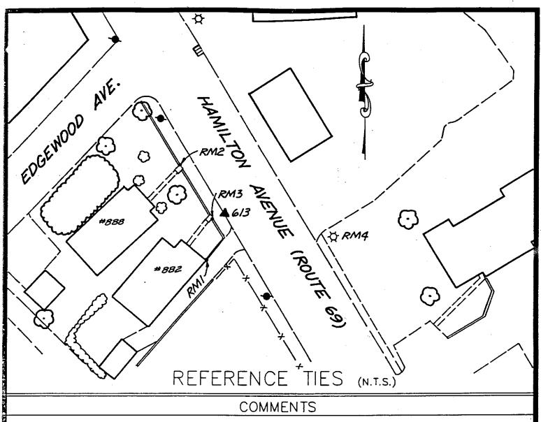
STATION #613: SET BRASS DISK IN TOP OF CONCRETE CURB ON WEST SIDE OF RTE. #69, 22.01±
