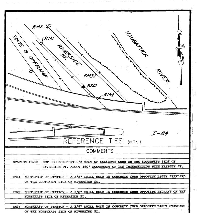
RM4: SOUTHEAST OF STATION - A 3/8" DRILL HOLE IN CONCRETE CURB OPPOSITE CONCRETE BRIDGE
