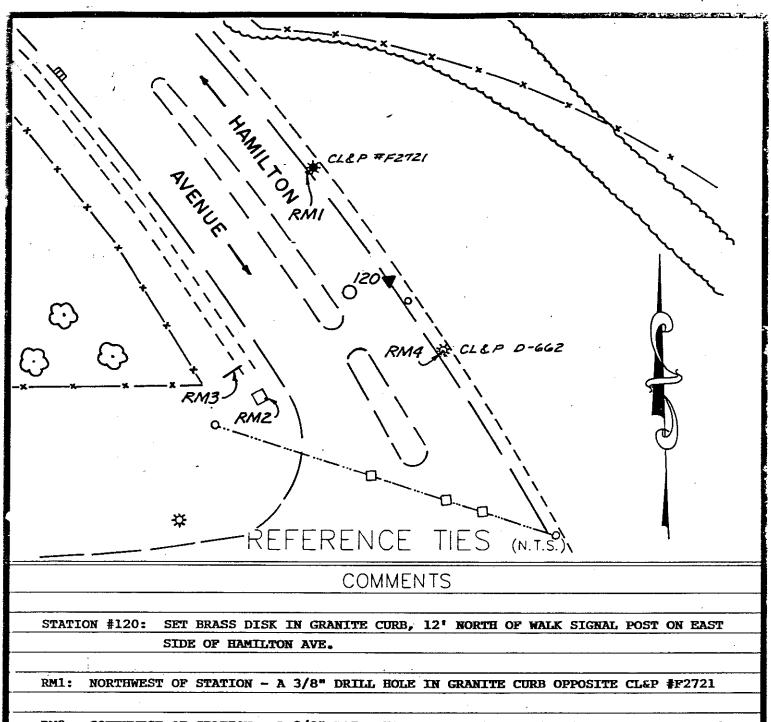
RM2: SOUTHWEST OF STATION - A 3/8" DRILL HOLE IN THE SOUTHEAST CORNER OF A CONCRETE BASE OF A TRAFFIC CONTROL BOX
