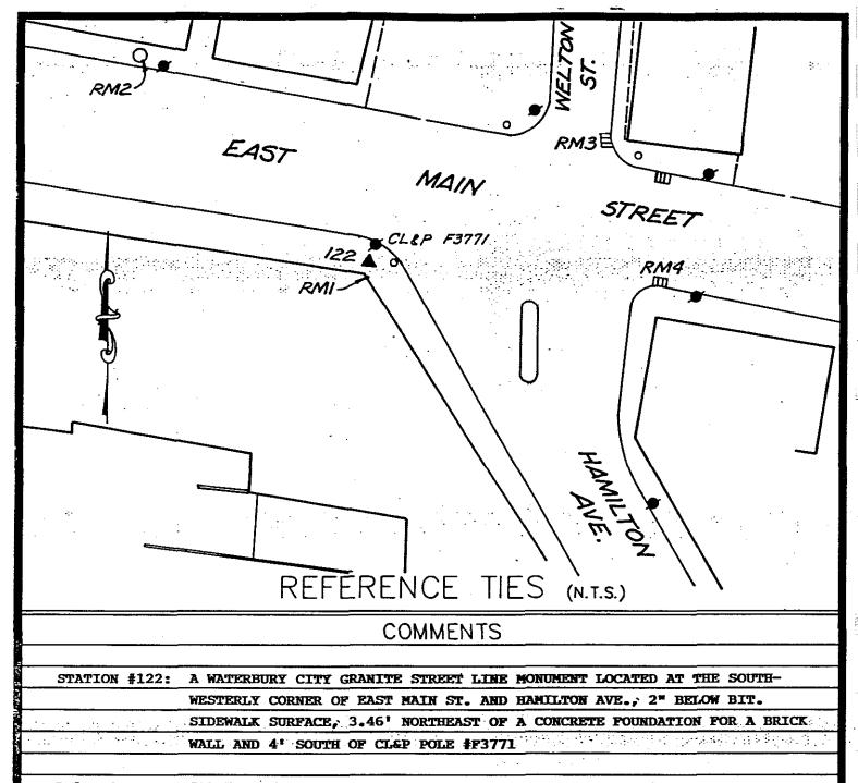
RM1: SOUTH OF STATION - A DRILL HOLE IN THE CONCRETE FOUNDATION OF BRICK WALL
