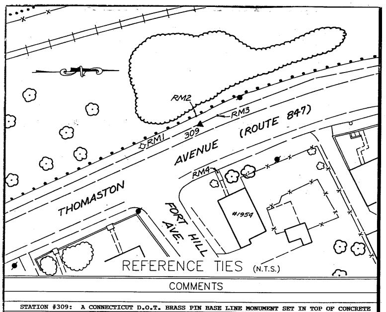
STATION #309: A CONNECTICUT D.O.T. BRASS PIN BASE LINE MONUMENT SET IN TOP OF CONCRETE
