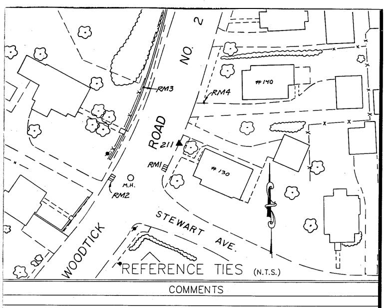
STATION #211: A BRASS DISK IN CONCRETE CURB, EAST SIDE OF WOODTICK RD., 65' NORTH OF SNET CO. POLE #5060
