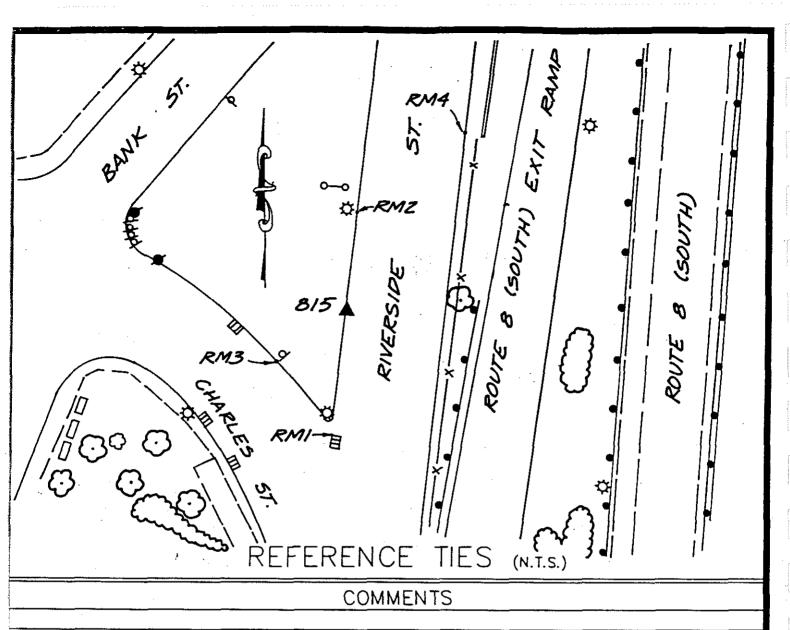
STATION #815: D.O.T. DISK IN CONCRETE CURB ON WEST SIDE OF RIVERSIDE ST. AND 50'± NORTH OF NORTHEAST EDGE OF CHARLES ST.
