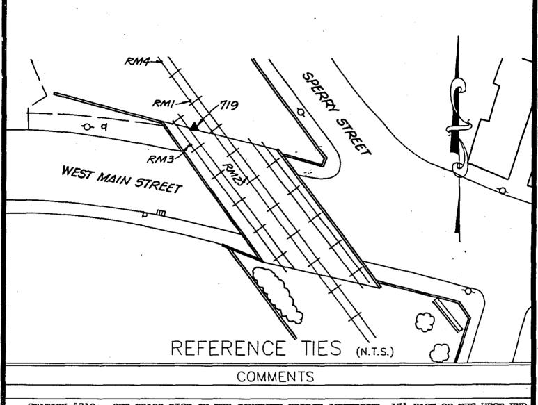
STATION #719: SET BRASS DISK ON THE CONCRETE BRIDGE ABUTTMENT, 17 EAST OF THE WEST END
