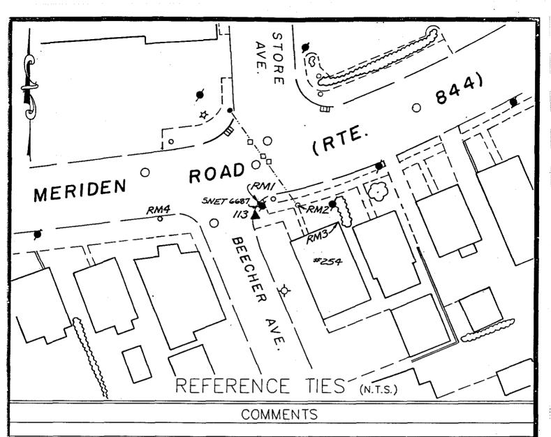
STATION #113: SET BRASS DISK IN TOP OF CURB OF HANDICAP RAMP, EAST SIDE OF BEECHER AVE.
