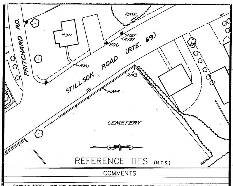
STATION #206: SET ROD MONUMENT IN BIT. WALK ON NORTH EDGE OF BIT. DRIVEWAY FOR HOUSE #311, 26' SOUTH OF SNET CO. POLE #10197, WEST SIDE OF THE ROAD
