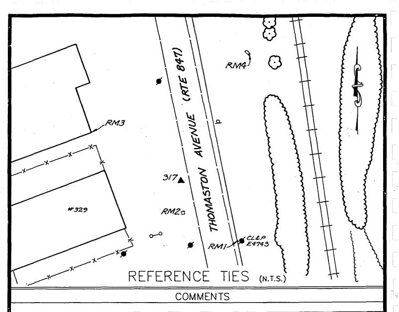
STATION #317: A CONNECTICUT D.O.T. BRASS DISK STAMPED C-3335 AND SET IN THE TOP OF A
