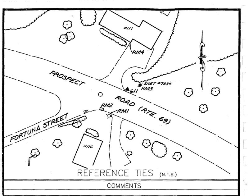
STATION #611: SET BRASS DISK IN STONE OUTCROP ON THE EAST SIDE OF RTE. #69, 3' EAST OF EDGE OF BIT. AND 2' SOUTH OF SOUTH RANGE OF HOUSE #111
