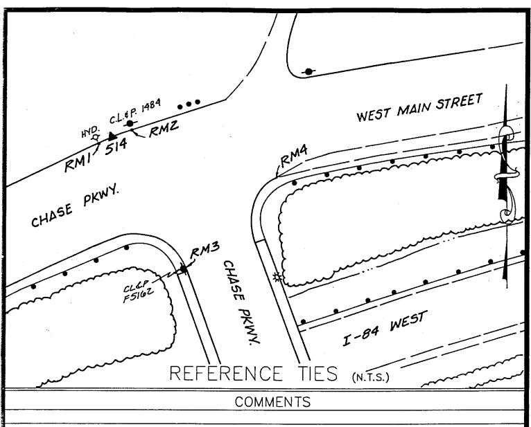
STATION #514: SET BRASS DISK IN CONCRETE CURB ON THE NORTH SIDE OF CHASE PARKWAY, 60°
