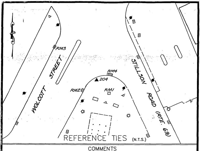
STATION #204: A CONNECTICUT GEODETIC SURVEY MONUMENT SET IN TOP OF A REINFORCED CONCRETE POST STAMPED 5823, 0.5° BEHIND BIT. WALK, 4° BELOW SURFACE OF THE GROUND, SOUTHWEST CORNER OF THE INTERSECTION OF WOLCOTT ST. AND STILLSON RD.
