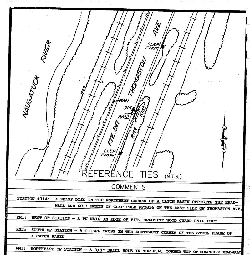
SOUTHEAST OF STATION - A 3/8" DRILL HOLE IN THE SOUTHWEST CORNER TOP OF CONCRETE
