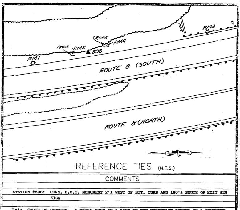
RM1: SOUTH OF STATION - A DRILL HOLE IN A BOLT IN THE NORTHEAST CORNER OF A CONCRETE LIGHT STANDARD BASE
