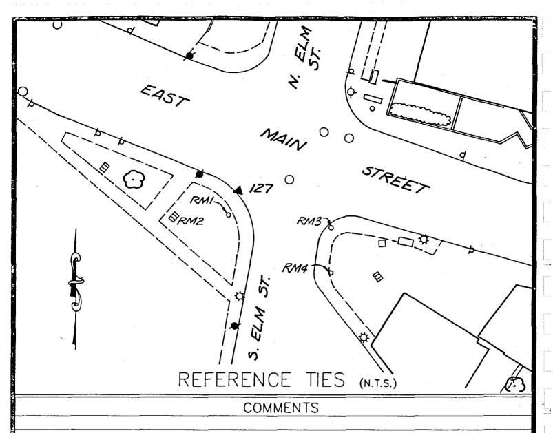
STATION #127: A PK NAIL IN THE PAVEMENT; 3'± NORTH OF GRANITE CURB OPPOSITE WEST END OF THE HANDICAP RAMP
