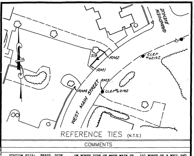
STATION #519: BRASS DISK ON NORTH SIDE OF WEST MAIN ST., 10' NORTH OF A WALL AND 55.5' WEST OF A CLEP POLE #62193S
