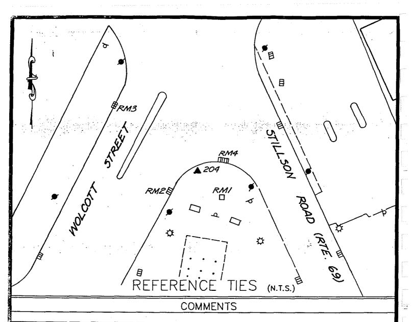
STATION #204: A CONNECTICUT GEODETIC SURVEY MONUMENT SET IN TOP OF A REINFORCED
