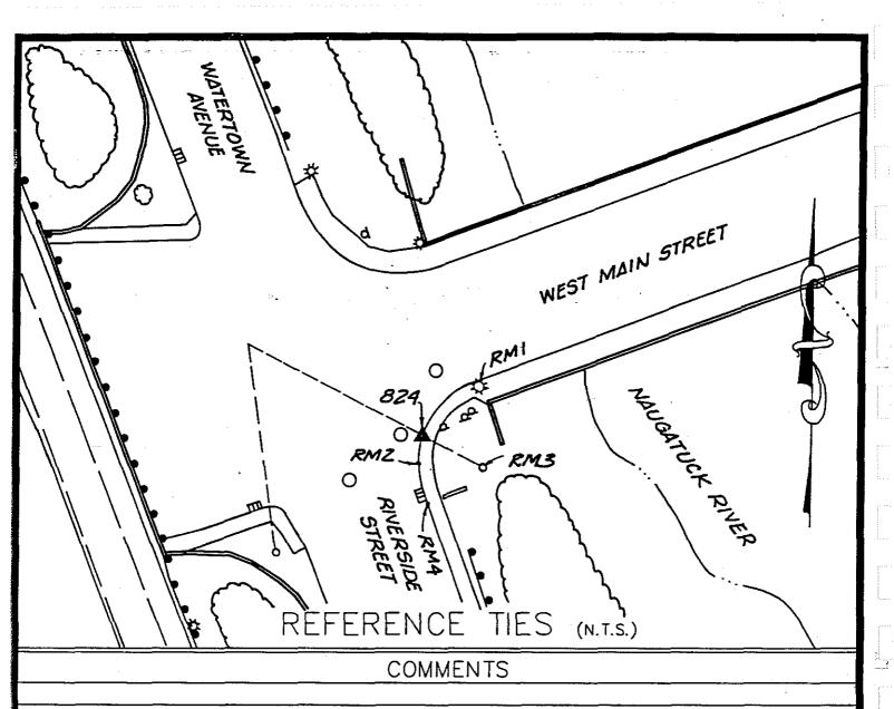
STATION #824: CONN. D.O.T. RANDOM DISK IN THE SIDEWALK 6' WEST OF FIRE CALL BOX, EAST SIDE OF RIVERSIDE ST. AND SOUTH SIDE OF WEST MAIN ST.
