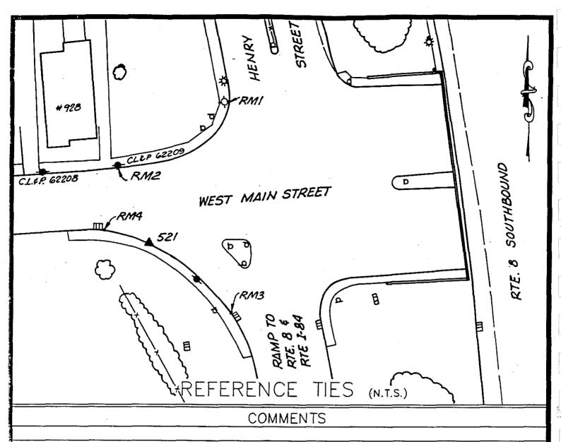
STATION #521: SET BRASS DISK IN CONCRETE CURB, SOUTH SIDE OF WEST MAIN ST., 25' EAST OF EAST RANGE OF HOUSE #928
