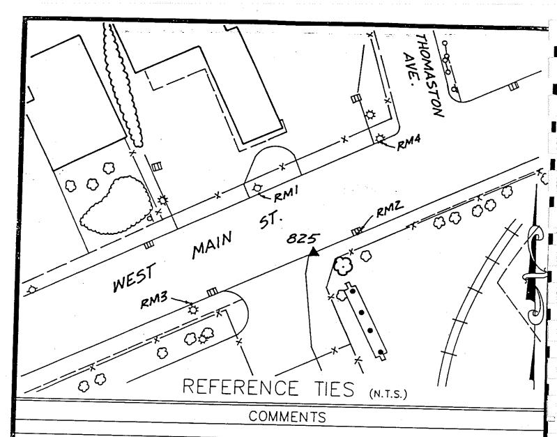
STATION #825: SET BRASS DISK IN CONCRETE CURB ON THE SOUTH SIDE OF WEST MAIN ST., 5' WEST OF EAST RANGE OF THE GAS STATION, 90'± WEST OF THE CENTERLINE OF THOMASTON AVE.
