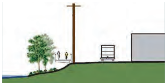
Due to topographical and floodway constraints, the trail will run on top of the existing retaining wall behind the Colonial Plaza Shopping Center.
